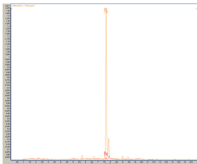
Fig. 1. MRM transitions of hydroxy-atenolol (283 > 178 and 283 > 107) at R_t = 7.65 min.
